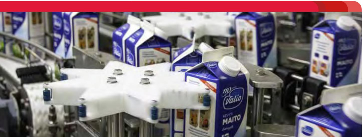
*The driven star wheel permits gentle and safe reorientation of bricks.*
